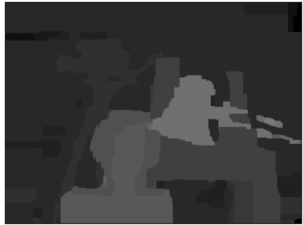
Figure 2: Disparity Depth Map resulting from naive belief propagation algorithm with Felzenszwalb optimizations for 5000 iterations
