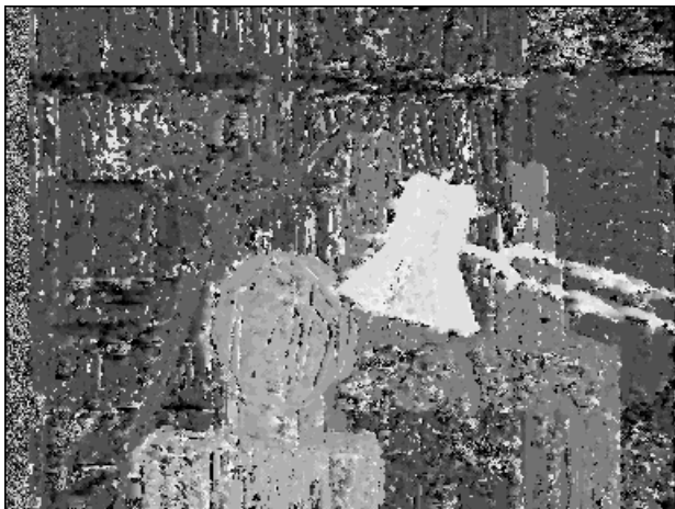
Figure 1: Disparity Depth Map resulting from naive belief propagation algorithm for 5000 iterations
